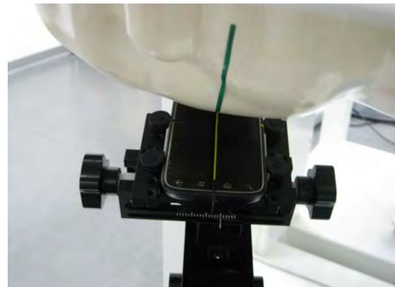
Fig.4 Right Head Section / Ear-Tilt Position(15°)
