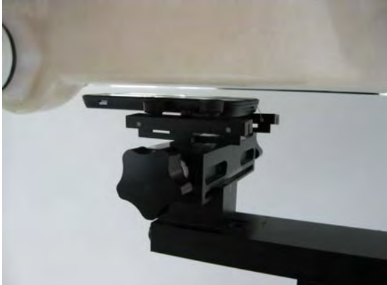
Fig.7 EUT front to flat phantom
