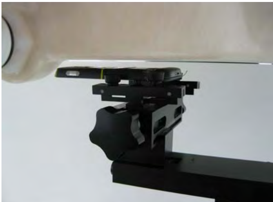
Fig.8 EUT rear to flat phantom
