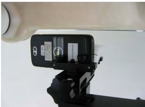
Fig.12 EUT Left to flat phantom
