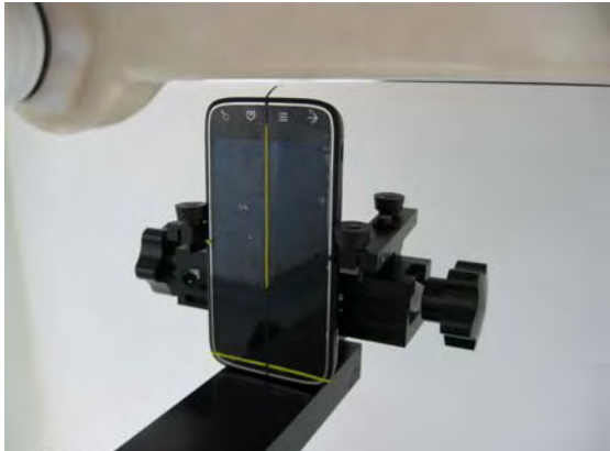
Fig.10 EUT Bottom to flat phantom
