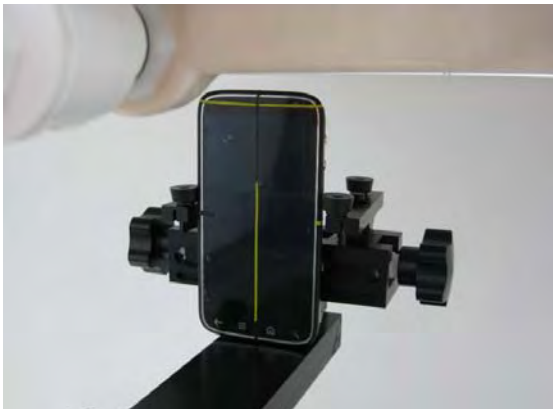
Fig.9 EUT Top to flat phantom
