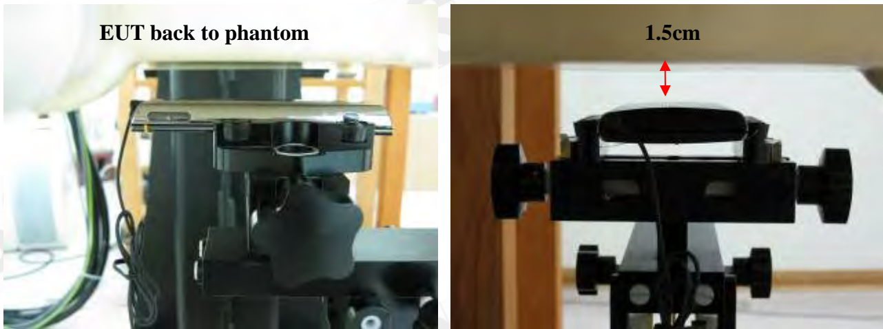
Fig.13 Body worn- EUT back to flat phantom and distance between flat phantom and mobile phone is 1.5 cm (repeated with headset)
