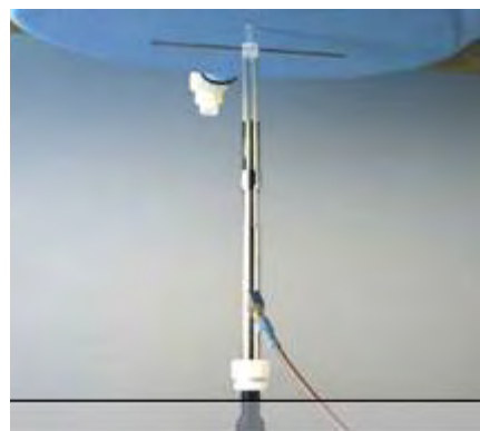
Photograph of the dipole Antenna
