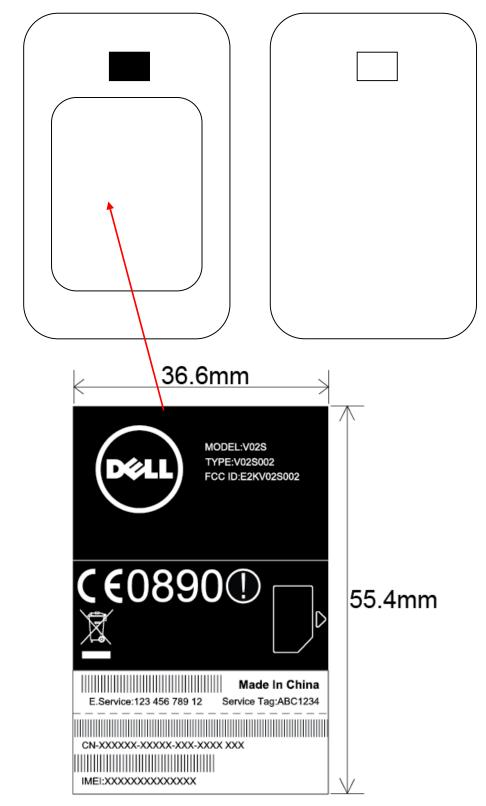
NOTE: label on internal PCB board, not on back cover
