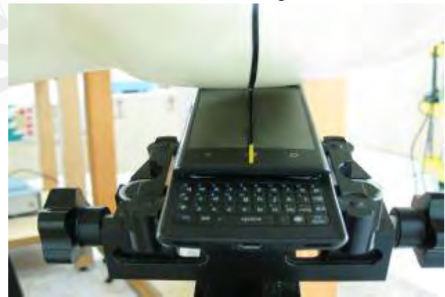
Fig.10 Left Head Section / Ear-Tilt Position(15°)_ Slider on
