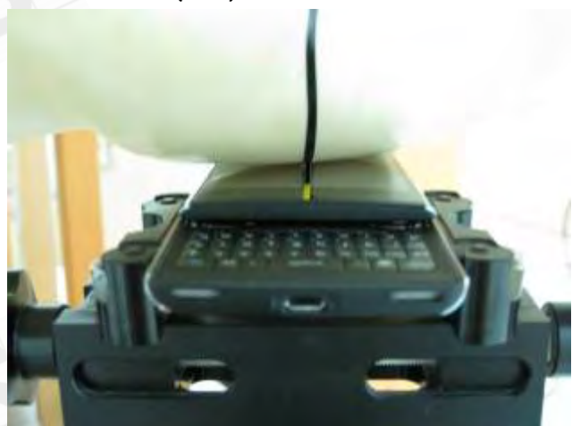
Fig.9 Left Head Section / Cheek-Touch Position_ Slider on
