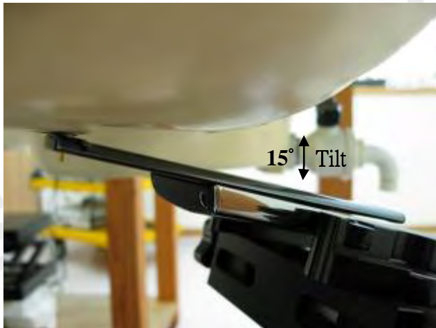
Fig.8 Right Head Section / Ear-Tilt Position(15°)_ Slider on
