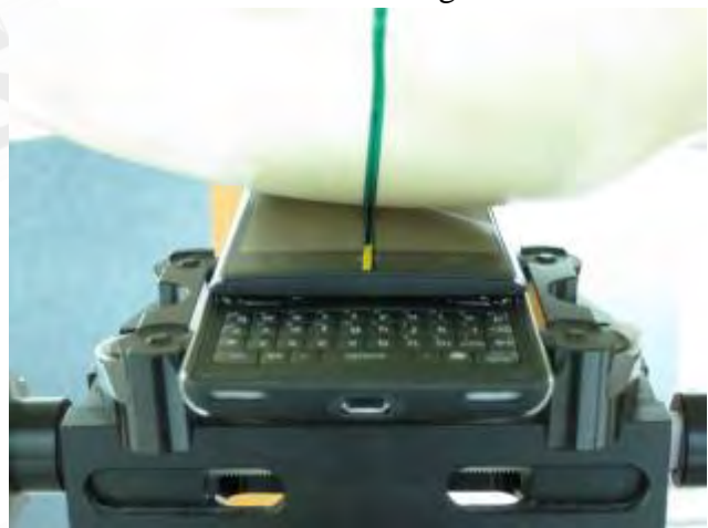
Fig.7 Right Head Section / Cheek-Touch Position_ Slider on
