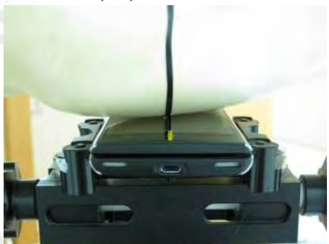
Fig.5 Left Head Section / Cheek-Touch Position_ Slider off
