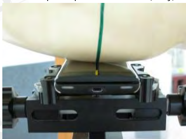
Fig.3 Right Head Section / Cheek-Touch Position_ Slider off
