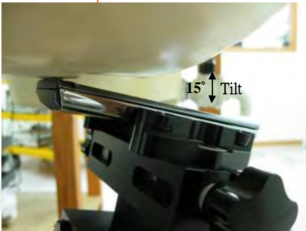
Fig.4 Right Head Section / Ear-Tilt Position(15°)_ Slider off
