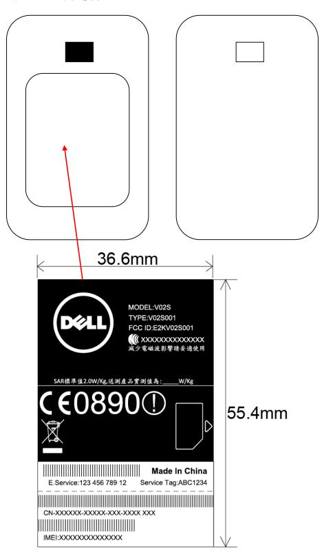
NOTE: label on internal PCB board, not on back cover
