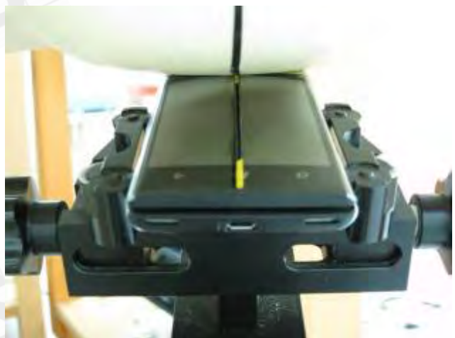
Fig.6 Left Head Section / Ear-Tilt Position(15°)_ Slider off
