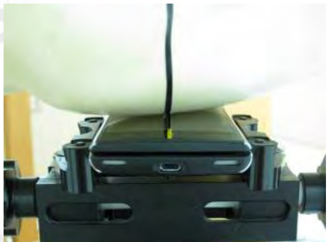
Fig.5 Left Head Section / Cheek-Touch Position_ Slider off
