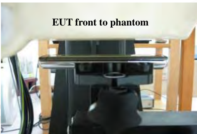
Fig.11 Body worn- EUT front to flat phantom and distance between flat phantom and mobile phone is 1.5 cm
