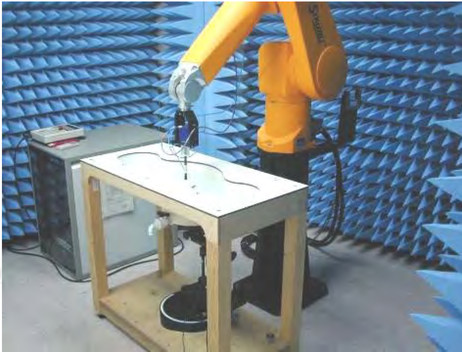
Fig.1 Photograph of the SAR measurement System
