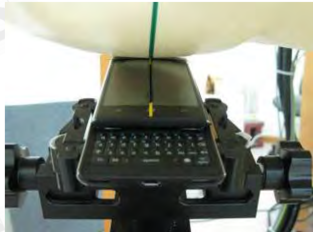
Fig.8 Right Head Section / Ear-Tilt Position(15°)_ Slider on
