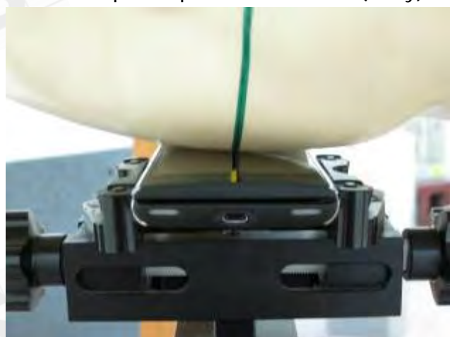
Fig.3 Right Head Section / Cheek-Touch Position_ Slider off
