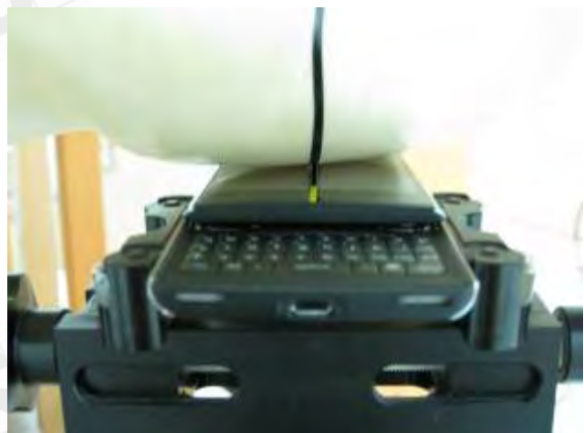
Fig.9 Left Head Section / Cheek-Touch Position_ Slider on
