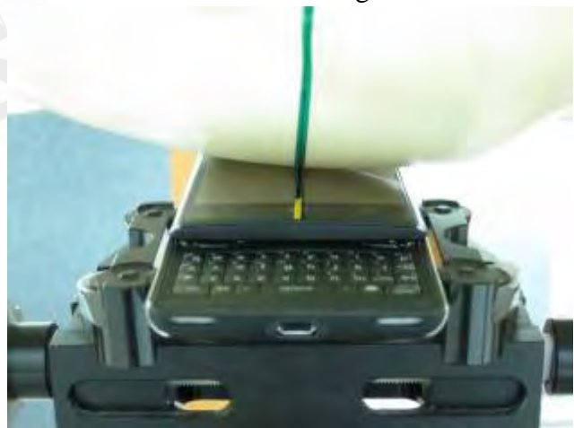
Fig.7 Right Head Section / Cheek-Touch Position_ Slider on
