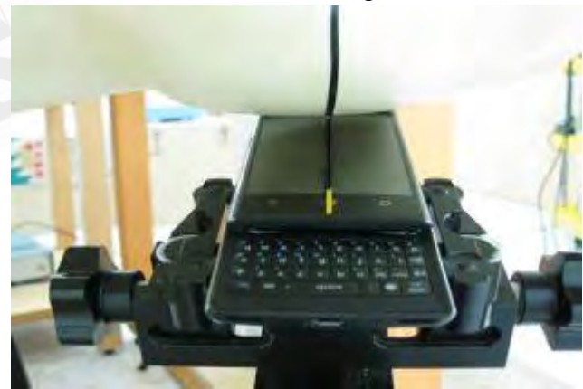
Fig.10 Left Head Section / Ear-Tilt Position(15°)_ Slider on
