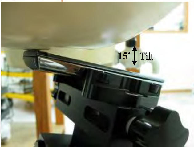
Fig.4 Right Head Section / Ear-Tilt Position(15°)_ Slider off
