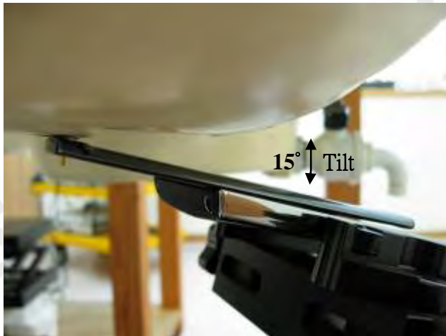
Fig.8 Right Head Section / Ear-Tilt Position(15°)_ Slider on
