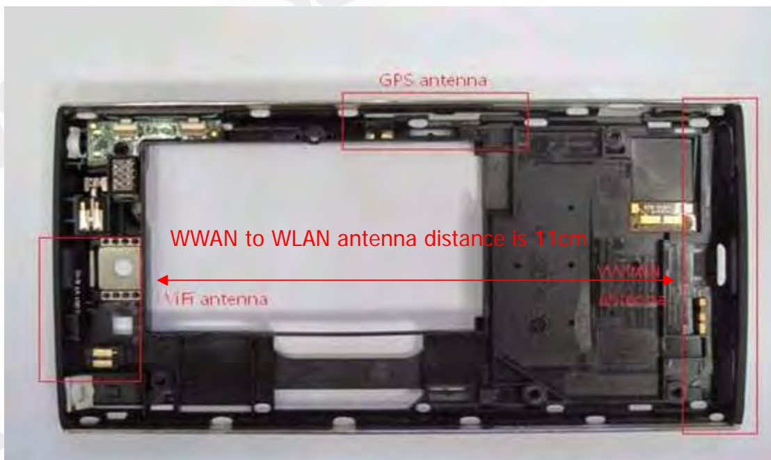
Fig.14 Antenna position of EUT
