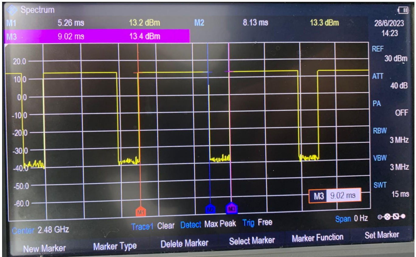
Time-domain plot for Bluetooth transmission signal
