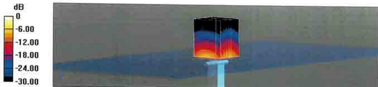
$$0 \text{ dB} = 13.4 \text{ W/kg} = 11.28 \text{ dBW/kg}$$
