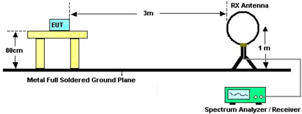
For radiated emissions from 30MHz to 1GHz
