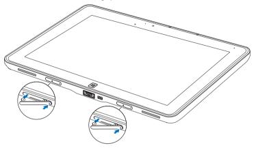
2 Align the power-adapter/docking port on the tablet with the 40-pin docking connector on the keyboard dock. Or, center the **Windows** button to the painted line on the front of the hinge holder.
