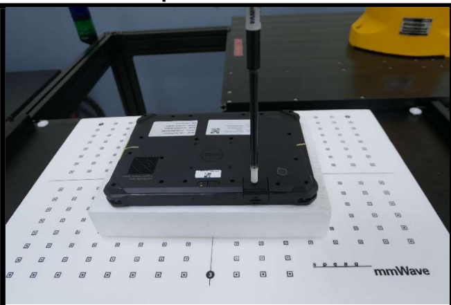
Rear Face of EUT Tested at 0mm
