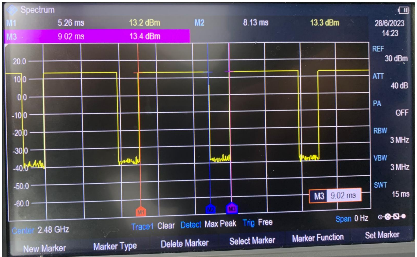
Time-domain plot for Bluetooth transmission signal
