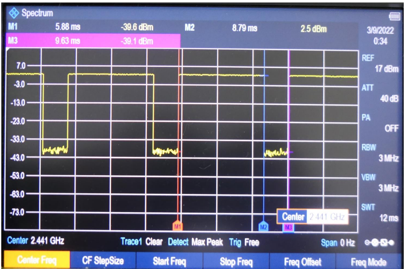
Time-domain plot for Bluetooth transmission signal
