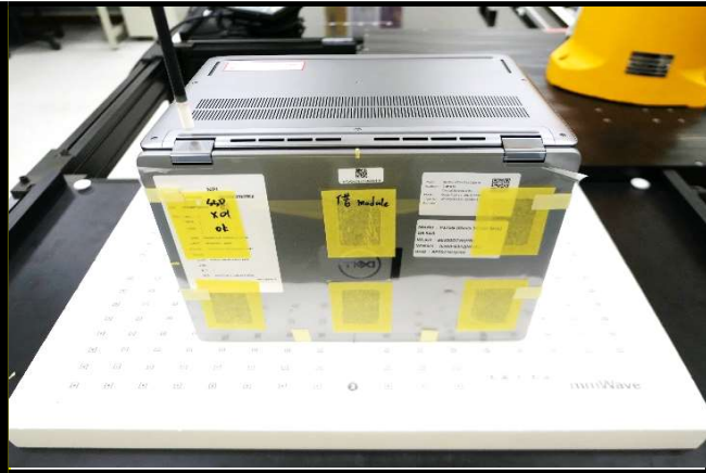
Bottom of Laptop Mode Tested at 0 mm
