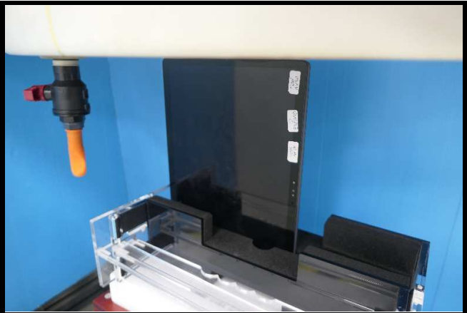
Left Side of Tablet Mode w RFID Tested at 0 mm
