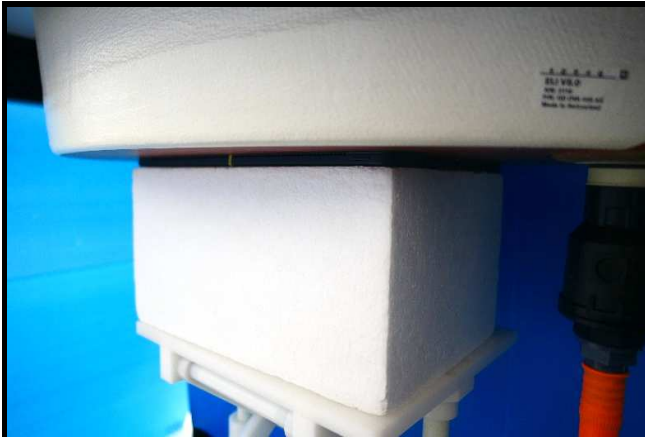
Rear Face of Tablet Mode wo RFID Tested at 0 mm
