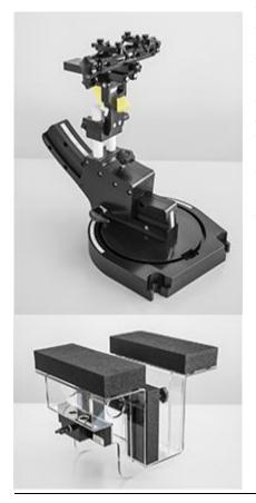
The DASY device holder is designed to cope with the different positions given in the standard. It has two scales for device rotation (with respect to the body axis) and device inclination (with respect to the line between the ear reference points). The rotation center for both scales is the ear reference point (ERP). Thus the device needs no repositioning when changing the angles.
