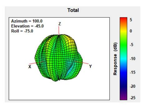
Max Antenna 3D Radiation Pattern 5470-5725 MHz
