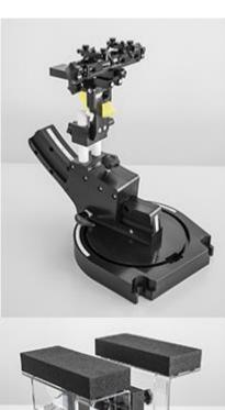
The DASY device holder is designed to cope with the different positions given in the standard. It has two scales for device rotation (with respect to the body axis) and device inclination (with respect to the line between the ear reference points). The rotation center for both scales is the ear reference point (ERP). Thus the device needs no repositioning when changing the angles.
