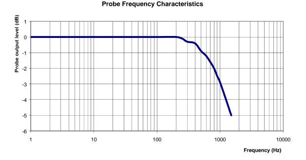
Video Bandwidth at 500 Hz1 dBVideo Bandwidth at 1.02 KHz:3 dB
