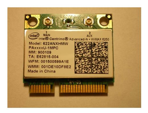
Photo showing label placement on half-mini card.
