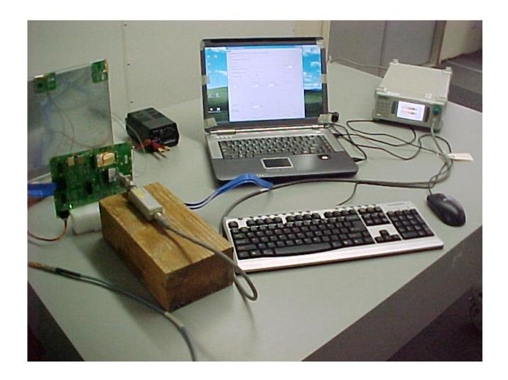
Maximum Peak Output Power Measurement Setup
