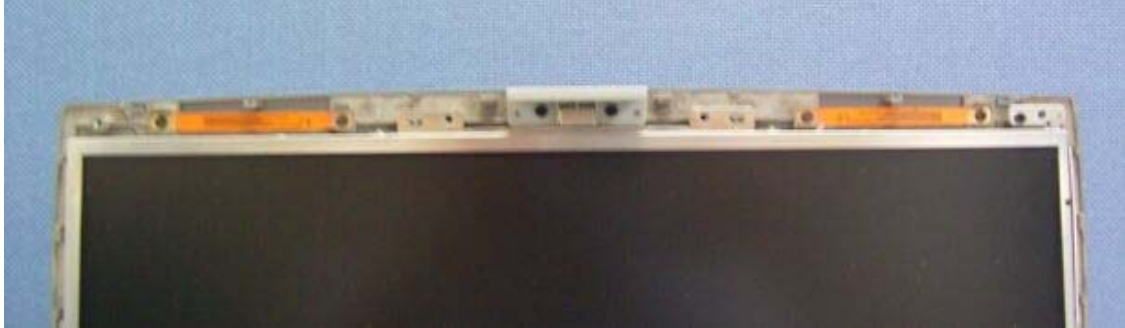
Picture of Antenna installed in the notebook
