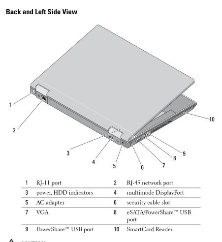
CAUTION: Do not block, push objects into, or allow dust to accumulate in the air vents. Do not store your Dell computer in a low-airflow environment, such as a closed briefcase, while it is running. Restricting the airflow can damage the computer or cause a fire. The computer turns on the fan when the computer gets hot. Fan noise is normal and does not indicate a problem with the fan or the computer.
