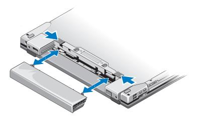
Remove the battery by sliding the battery tabs inward and moving the battery away from the notebook. Install the battery by pushing the battery inward until it clicks into place.
