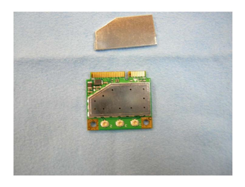
Top View "Top Shielding removed"
