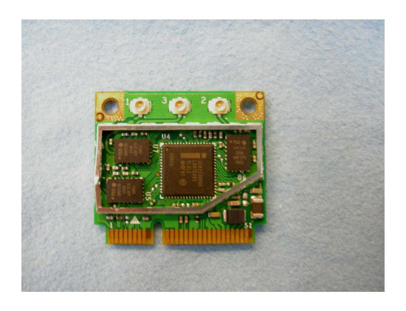
Top View "Inner Shielding removed"
