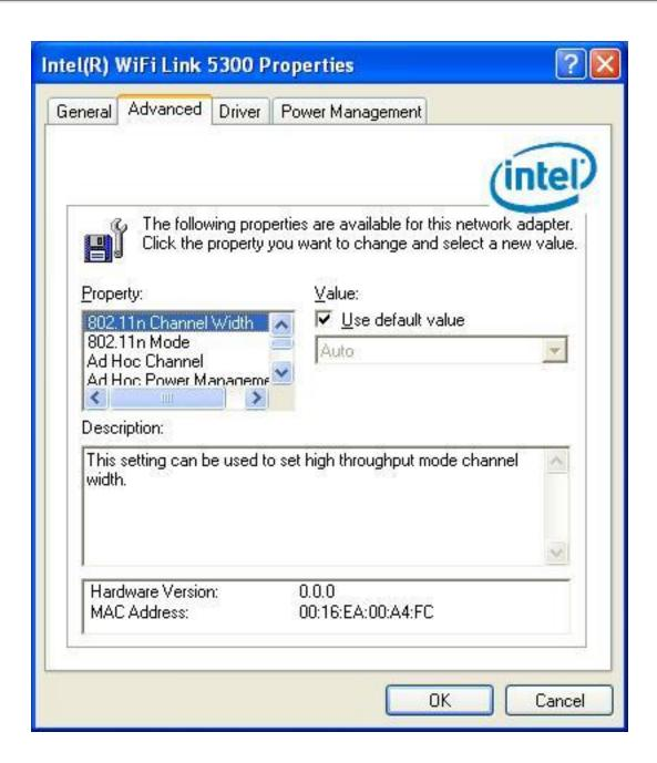
The Adapter Settings, advanced tab, displays the device properties for the wireless adapter installed on your computer.
