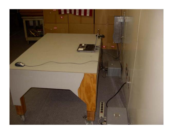
AC Conducted Emissions Measurement (Rear View) Setup
