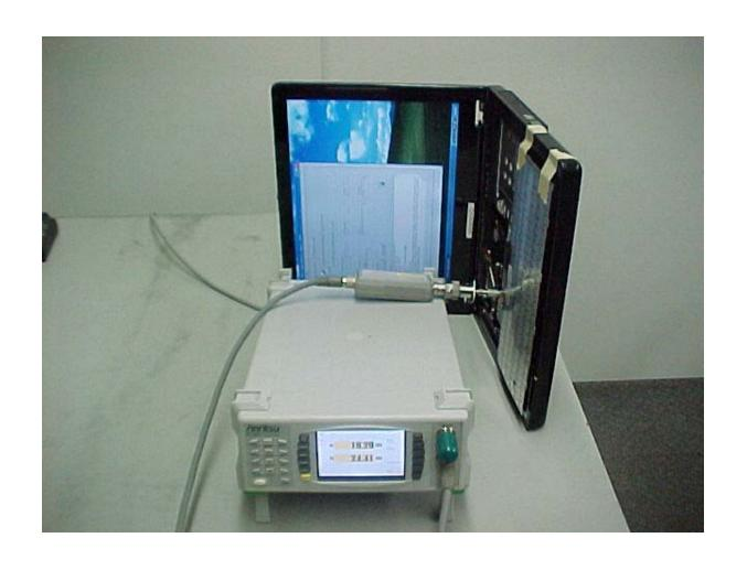
Maximum Peak Output Power Measurement Setup
