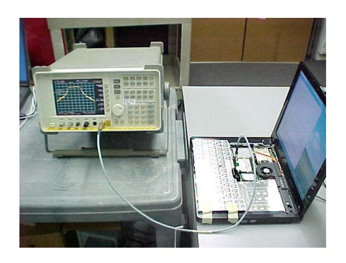
Conducted Emissions at Antenna Terminal Setup
