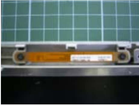
Picture of Antenna installed in the notebook
