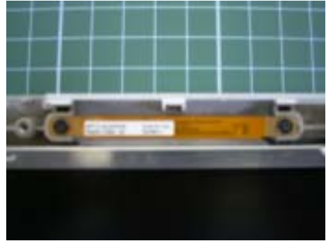
Picture of Antenna installed in the notebook
