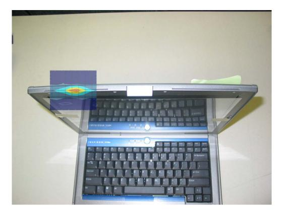
1 gram SAR Value 10 gram SAR Value Area Scan Peak SAR Zoom Scan Peak SAR : X = 13.10 Y = -62.20 Z = 2.8 Value = 0.50 W/kg : X = 13.10 Y = -62.20 Z = 2.8 Value = 0.30 W/kg : 0.73 : 1.07
