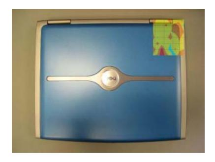
1 gram SAR Value :  $X = -2.10 \ Y = 29.80 \ Z = 0.2 \ Value = 0.34 \ W/kg$  10 gram SAR Value :  $X = -2.10 \ Y = 29.80 \ Z = 0.2 \ Value = 0.30 \ W/kg$
