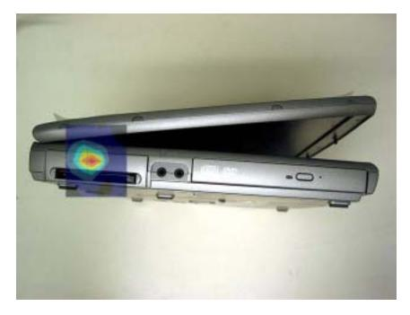
1 gram SAR Value :  $X = 8.10 \ Y = -0.20 \ Z = 0.3 \ Value = 0.72 \ W/kg$  10 gram SAR Value :  $X = 8.10 \ Y = -0.20 \ Z = 0.3 \ Value = 0.36 \ W/kg$
