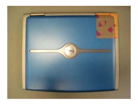
1 gram SAR Value :  $X = 28.50 \ Y = 9.90 \ Z = 1.6 \ Value = 0.30 \ W/kg$ 10 gram SAR Value :  $X = 28.50 \ Y = 9.90 \ Z = 1.6 \ Value = 0.29 \ W/kg$
