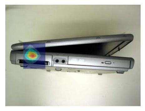
1 gram SAR Value :  $X = 8.00 \ Y = -0.30 \ Z = 0.6 \ Value = 0.53 \ W/kg$  10 gram SAR Value :  $X = 8.00 \ Y = -0.30 \ Z = 0.6 \ Value = 0.28 \ W/kg$
