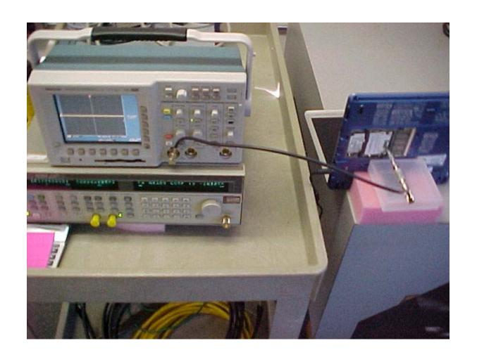
Maximum Peak Output Power Measurement Setup
