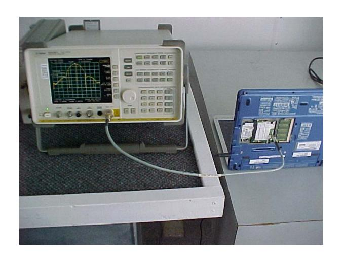
Conducted Emissions at Antenna Terminal Setup
