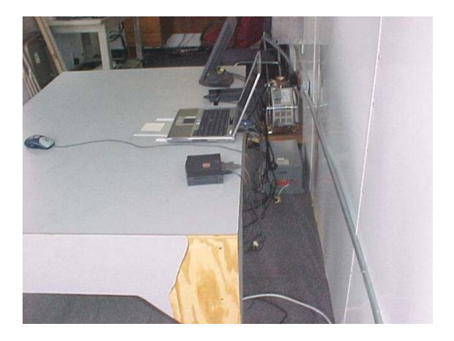
AC Conducted Emissions Measurement (Rear View) Setup
