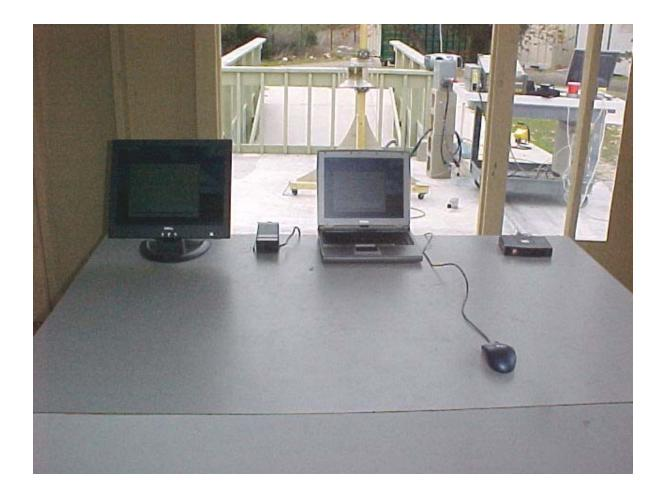
Radiated Emissions Measurement (30-1000 MHz) (Front View) Setup
