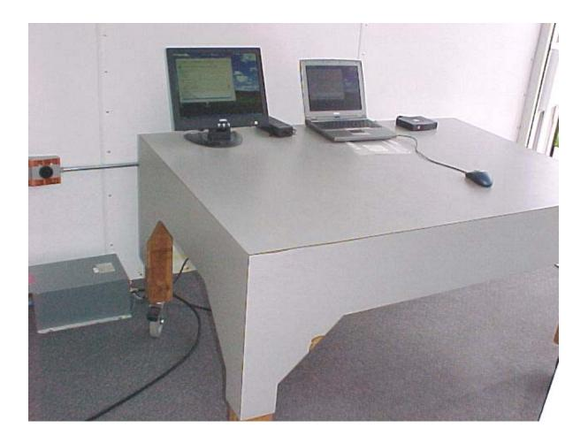
AC Conducted Emissions Measurement (Front View) Setup
