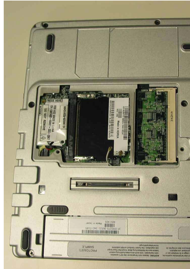
Bottom View showing the MINI PCI expansion slot with (left) and without (right) Wireless LAN Card installed
