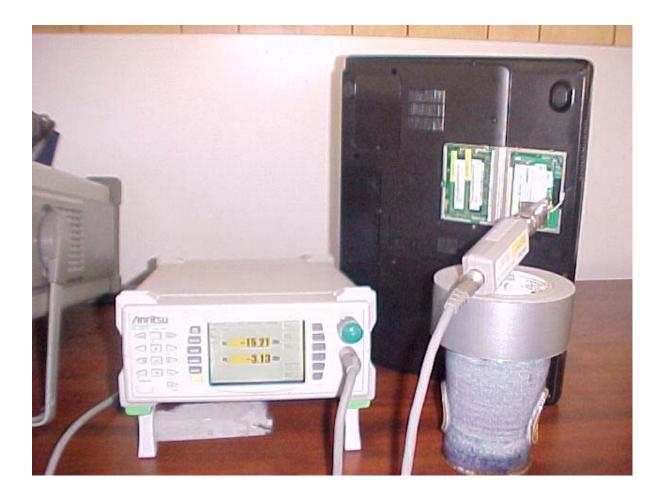
Maximum Peak Output Power Measurement Setup
