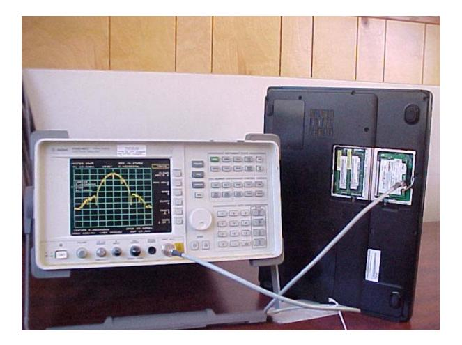
Conducted Emissions at Antenna Terminal Setup
