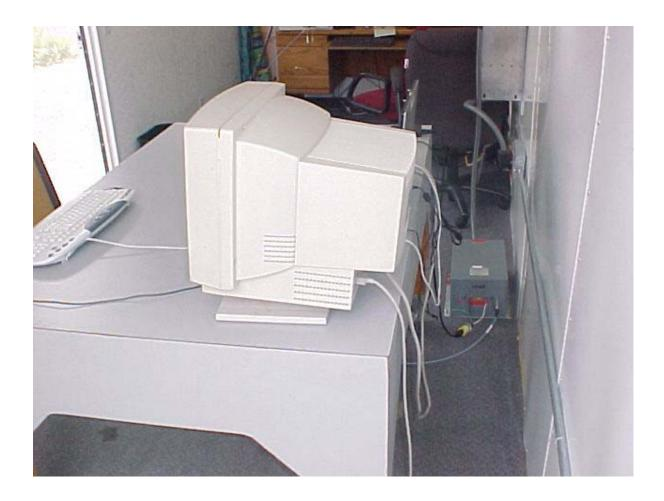
AC Conducted Emissions Measurement (Rear View) Setup
