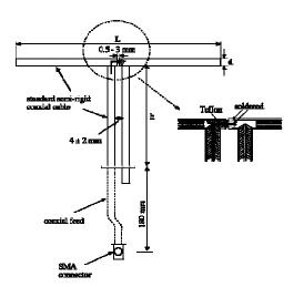
APREL Laboratories have developed frequency dipoles based on current scientific research carried both experimentally numerically here at the APREL Laboratories site. Mechanical and electrical parameters for the dipoles have been established experimental and numerical techniques, and target SAR values have been established following IEC methodologies. The results of the experimental and numerical research have been published and released for peer review.
