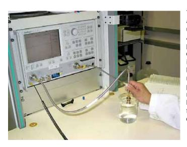
Tissue used during the SAR assessment is calibrated prior to use in the measurement process. APREL Laboratories use the co-axial probe method for all tissue calibration exercises. Tissue which is being used over a period of 24 hours is re-calibrated to ensure that change to the dielectric properties will affect the SAR measurement process. The table below provides details of the results from the tissue equivalent dielectric calibration.
