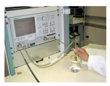
Tissue used during the SAR assessment is calibrated prior to use in the measurement process. APREL Laboratories use the co-axial method for all tissue probe calibration exercises. Tissue which is being used over a period of 24 hours is re-calibrated to ensure that change to the dielectric properties will affect the SAR measurement process. The table below provides details of the results from the tissue equivalent dielectric calibration.
