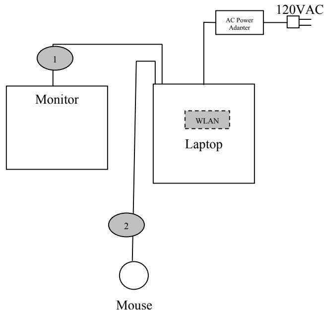
Cable 1: This is a 6-foot braid and foil shielded round cable connecting the Latitude | D610 Notebook Computer with the Dell LCD monitor. It has metallic DB-15 type connector at the computer end and is hardwired to the monitor. The cable is bundled to a length of one meter and the shield of the cable is grounded to the chassis of both devices via the connector shells.
