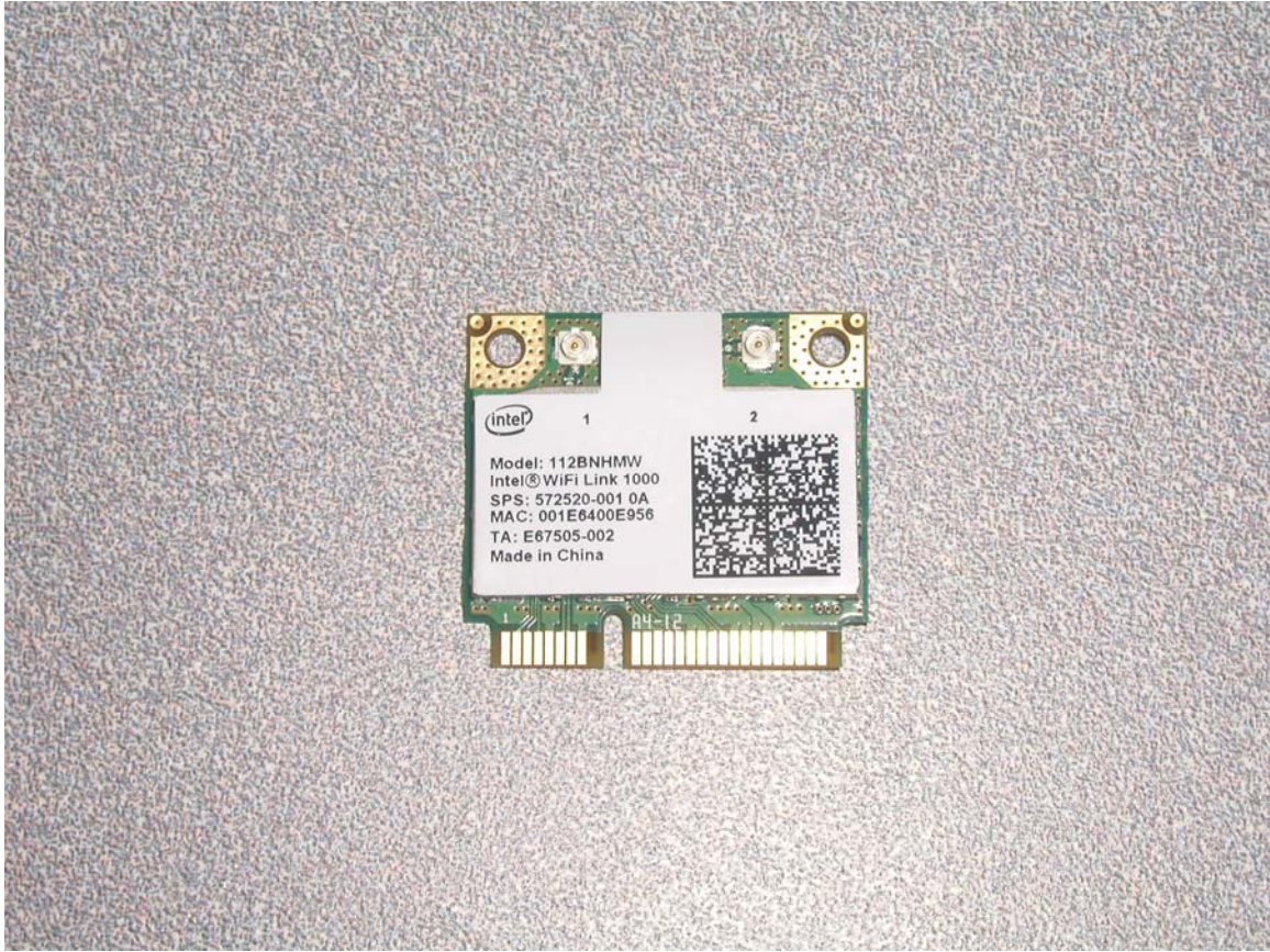
Photo shows label placement on half-mini card. Label wraps around onto other side of the board.
