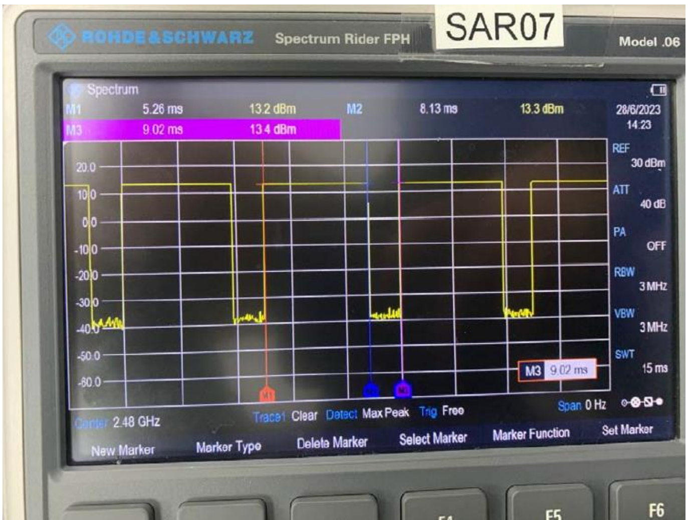
Time-domain plot for Bluetooth transmission signal
