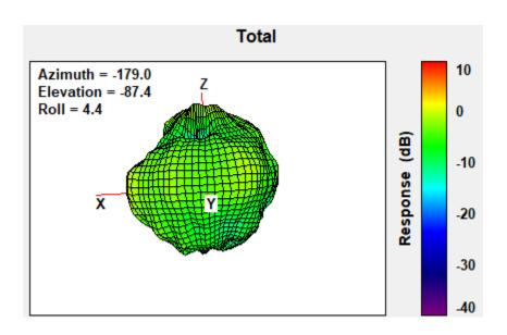
Max Antenna 3D Radiation Pattern 5850-5895 MHz
