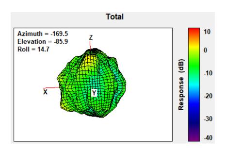
Max Antenna 3D Radiation Pattern 5850-5895 MHz
