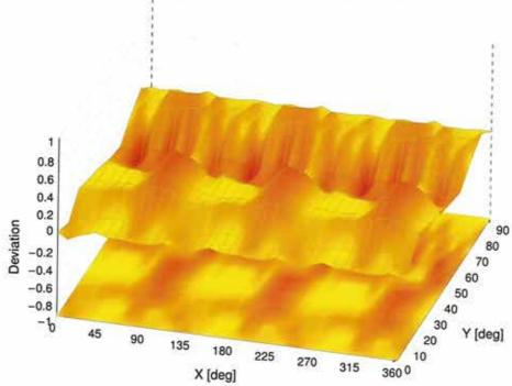
60GHz: 3D isotropy, E-field parallel to probe axis
