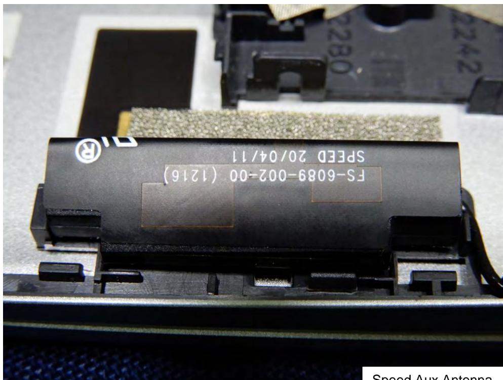
Speed Aux Antenna Part No. 025.901MP.0001
