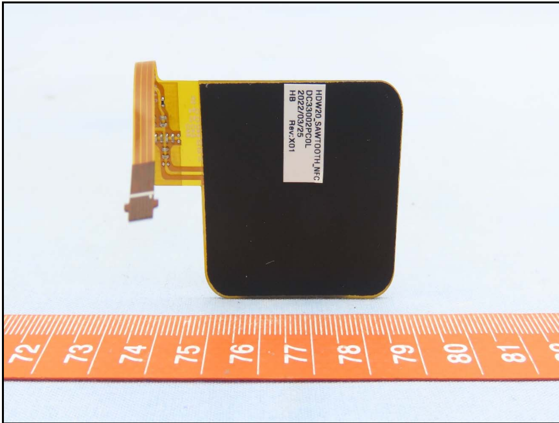
Loop Antenna (Brand: Hong.Bo, Model: 1FP3J (DC33002PC0L))
