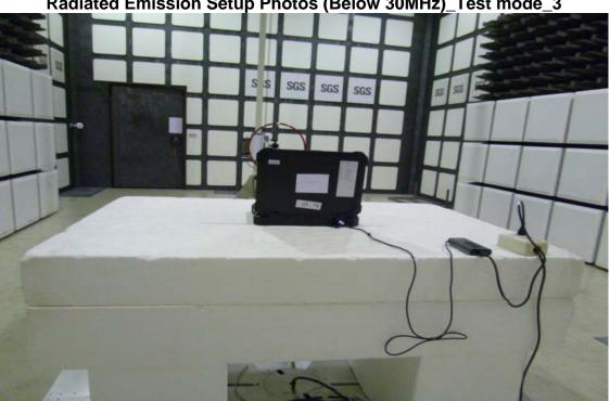
Radiated Emission Setup Photos (Below 30MHz)\_Test mode\_3
