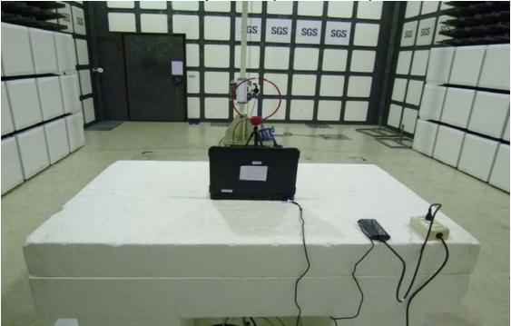
Radiated Emission Setup Photos (Below 1GHz)
