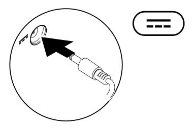
WARNING: The AC adapter works with electrical outlets worldwide. However, power connectors and power strips vary among countries. Using an incompatible cable or improperly connecting the cable to a power strip or electrical outlet may cause fire or permanent damage to your computer.
