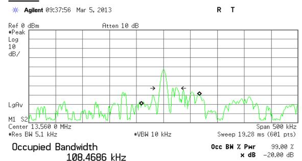
Transmit Freq Error 13.132 kHz x dB Bandwidth 32.861 kHz
