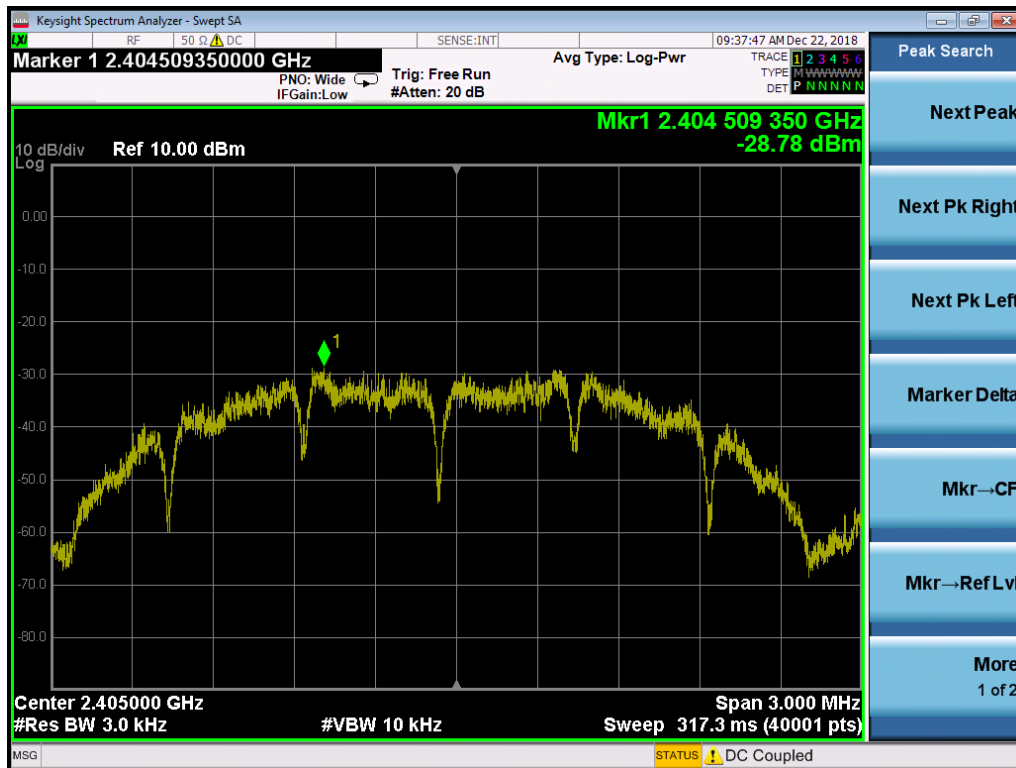
Power Spectral Density, Low Channel
