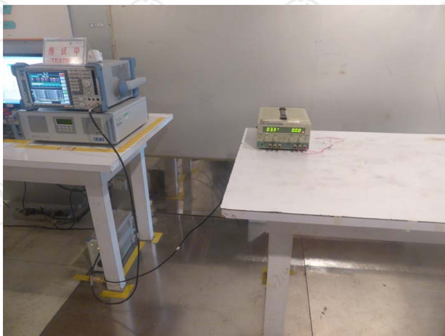
TEST SETUP OF CONDUCTED EMISSION
