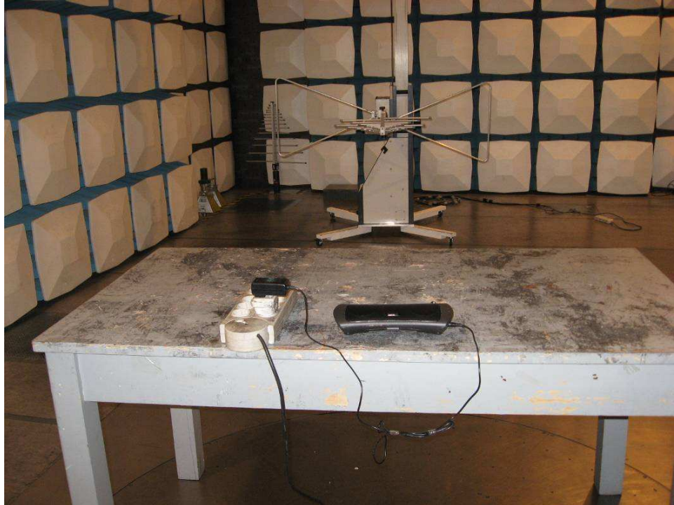
Photograph 6: Set-up for Spurious Emissions (1GHz-18GHz)
