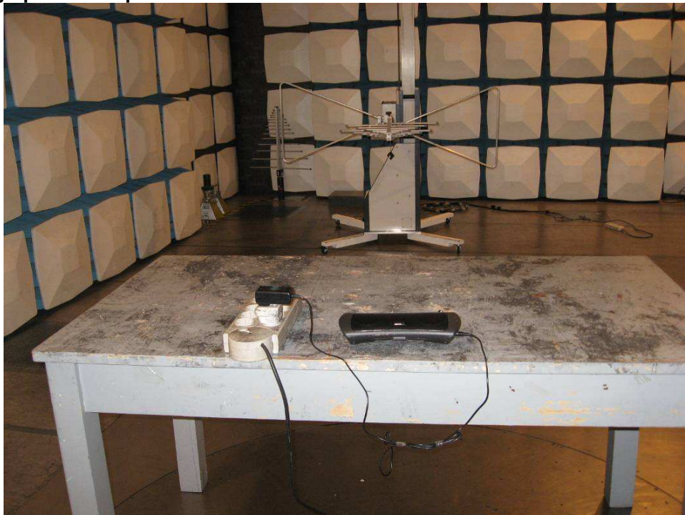
Photograph 2: Set-up for Radiated Emissions
