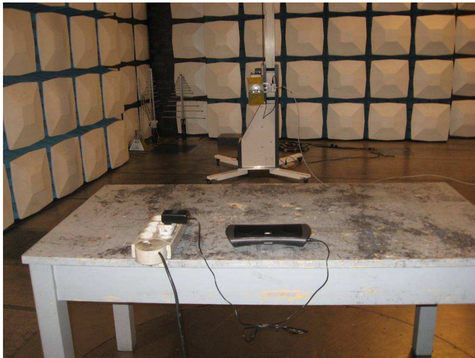
Photograph 6: Set-up for Spurious Emissions (1GHz-18GHz)
