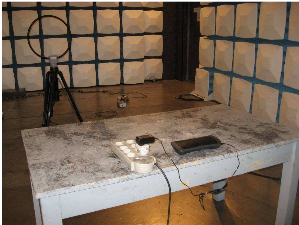
Photograph 4: Set-up for Spurious Emissions (9kHz-30MHz)
