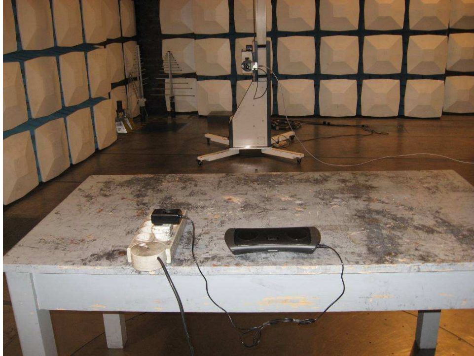
Photograph 7: Set-up for Spurious Emissions (18GHz-26GHz)
