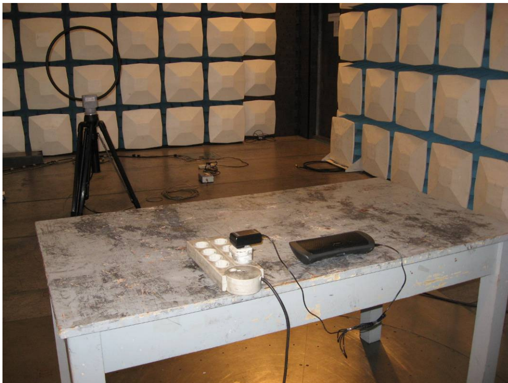
Photograph 4: Set-up for Spurious Emissions (9kHz-30MHz)
