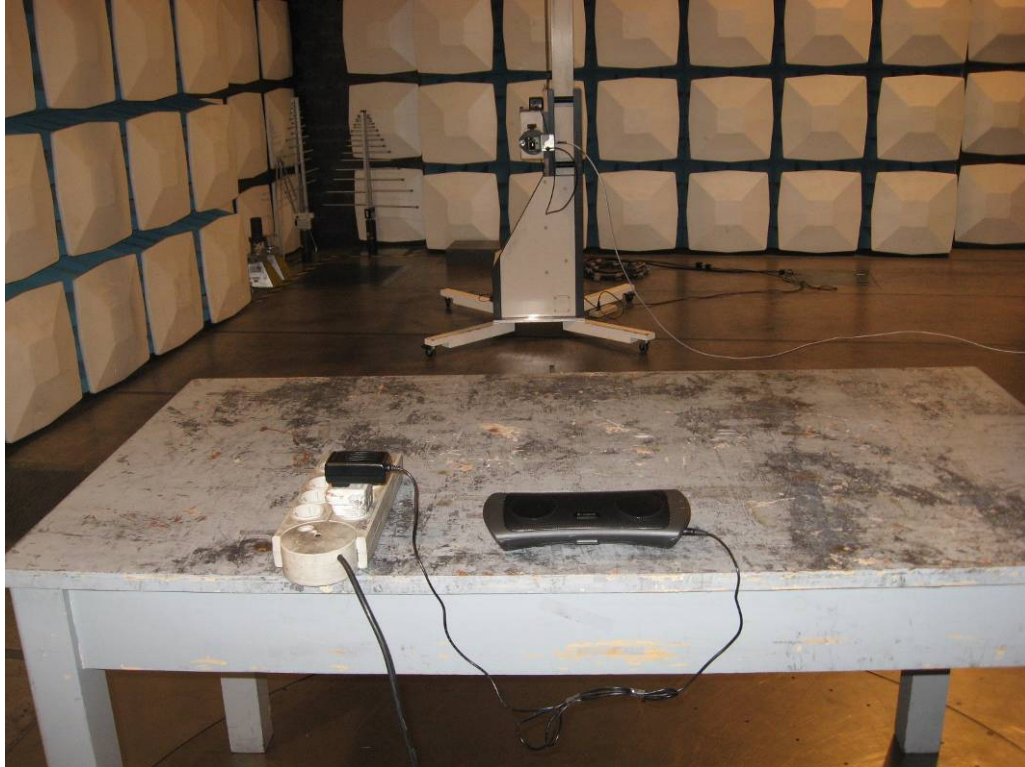
Photograph 7: Set-up for Spurious Emissions (18GHz-26GHz)
