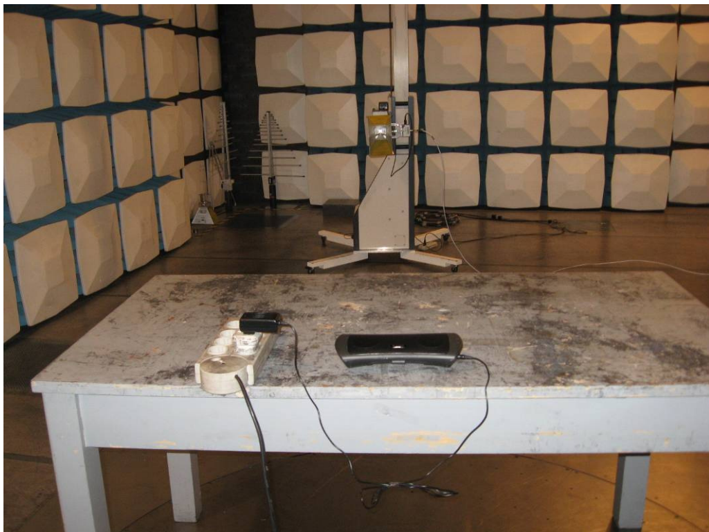
Photograph 6: Set-up for Spurious Emissions (1GHz-18GHz)
