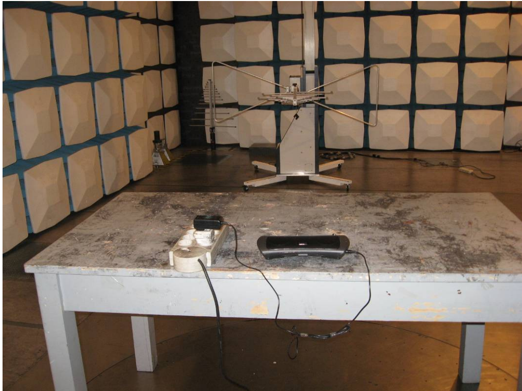
Photograph 6: Set-up for Spurious Emissions (1GHz-18GHz)
