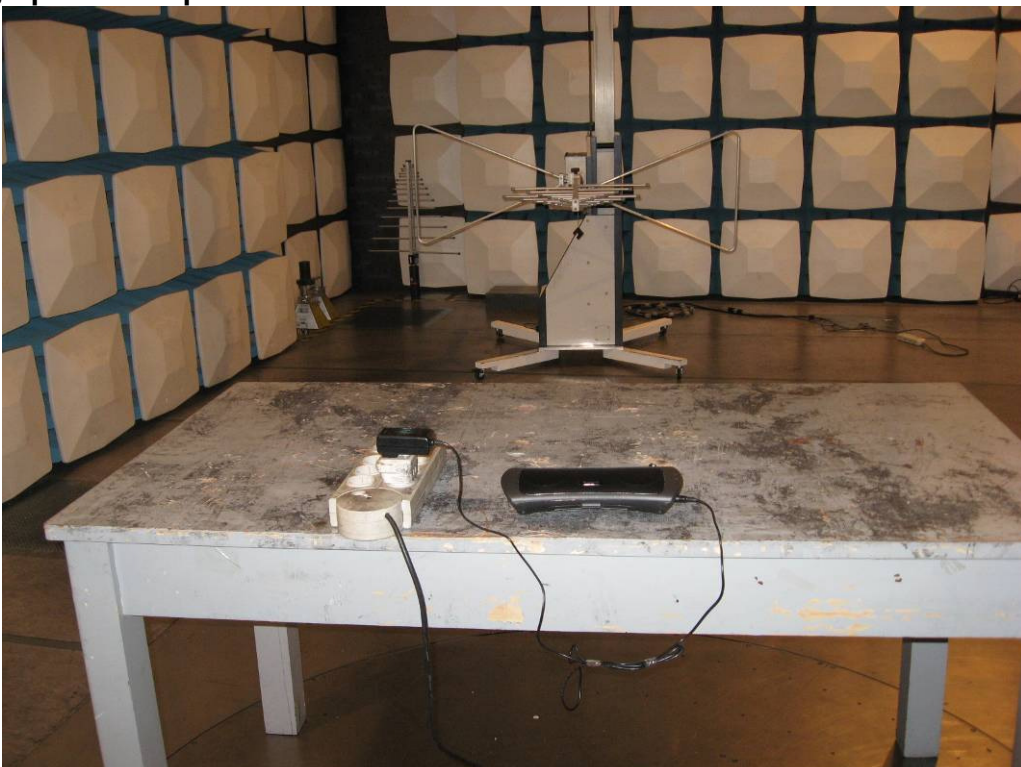
Photograph 2: Set-up for Radiated Emissions
